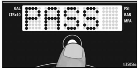
**NOTE:** If the knob is not aligned correctly, **FAIL** displays, then **KNOB** displays again. Ensure the Pressure Control Knob is aligned correctly, then try the calibration procedure again.
