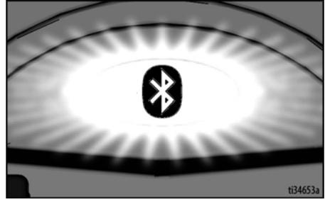
Blinking red LED total count equals the error code (for example: two blinks equals CODE 02).
