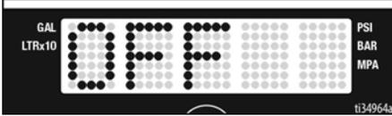
8. Short press **DISPLAY** button to move to WatchDog sensitivity menu. Press and hold **DISPLAY** button and Watchdog can be set to low, medium, or high sensitivity. Release **DISPLAY** button when desired sensitivity setting is displayed. Default is medium.
